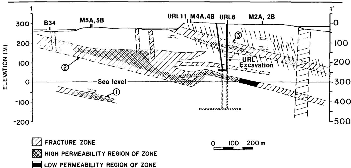
Figure 9 Cross section showing fracture zones in the rock mass containing the URL.
