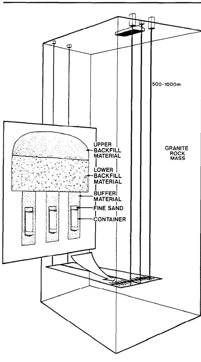
Figure 5 The Canadian concept for a nuclear fuel waste disposal vault.
