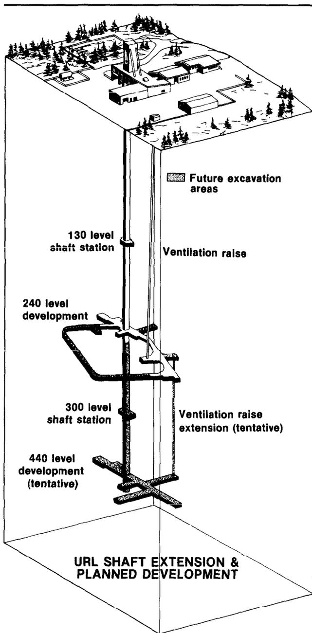
Figure 12 Schematic of the Underground Research Laboratory.
