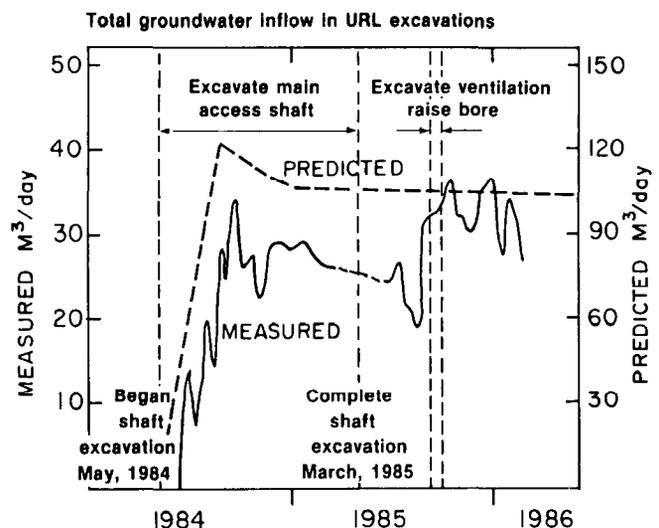
Figure 10 Comparison of predicted and measured groundwater inflow into the URL shaft.
