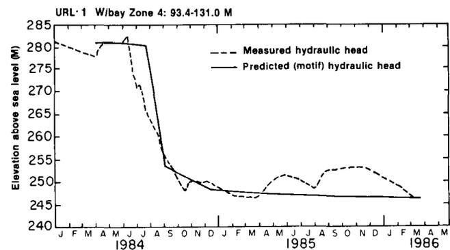
Figure 11 Comparison of predicted and measured hydraulic head of borehole URL-1 in the upper fracture zone.
