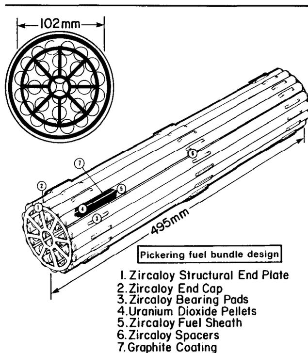
Figure 3 A typical CANDU fuel bundle assembly.
