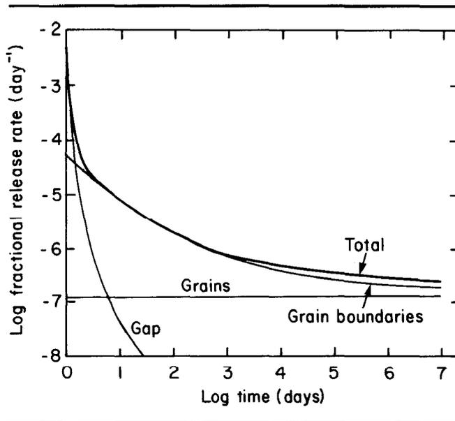
Figure 6 Release of radionuclides from CANDU fuel.
